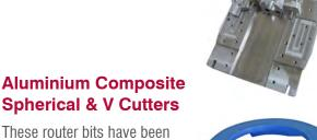
These router bits have been designed for machining aluminium composite materials (ACM). The V cutters have a 3mm flat tip to allow for a correct bend clearance.
