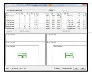
The **PANELBuilder** programming software provides an intuitive graphical interface for scheduling jobs to be cut on each of the virtual zones.
