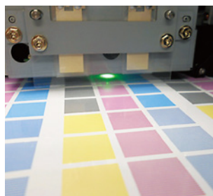
RGB sensor reads this difference to decide most appropriate correction value automatically
