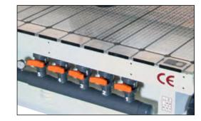
The innovative design of the aluminium vacuum bed allows zoned areas to be opened or closed as needed. This allows materials to be held as securely as possible and eliminates problems caused by movement while cutting.
