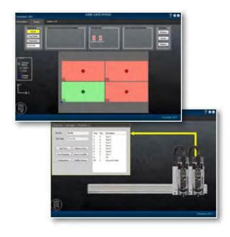
The A2MC Enterprise provides a powerful and easy to use graphical interface for setting up and monitoring your machine. Using a series of Windows-based apps it has been designed to help you get the best performance from your CNC router.
