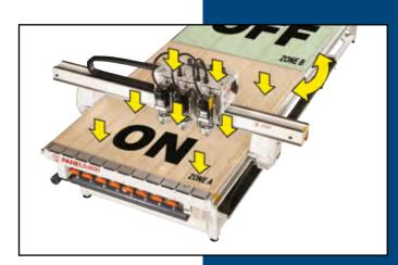
For applications that need a greater vertical clearance such as mould making or three dimensional carving, the standard 150mm gantry height can be extended to 250mm, 300mm or even greater.
