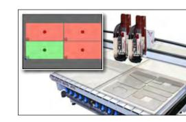
Auto zone management allows the router to operate in Live Deck mode which will automatically activate and deactivate zones according to the live position of the cutting head.
