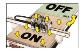
Pendulum Processing mode allows continuous production on two virtual beds. Eliminate machine downtime in between jobs to achieve up to twice the productivity.
