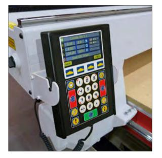
The AXYZ SmartConsole brings unprecedented ease of use, context sensitive menus, real-time display of machine status in addition to many more time-saving, functional and productivity features. It provides a graphical preview and current status of a running job and allows program feeds and speeds to be changed without pausing the program.
