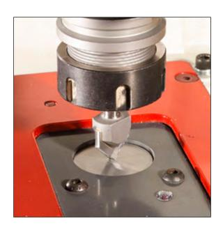
The tool-length sensor is used to automatically measure the length of a tool and create an accurate tool-length offset. This time-saving feature also ensures precise and consistent cutting depths with all tools.
