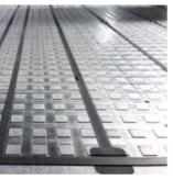
The innovative design of the aluminium vacuum bed allows zoned areas to be opened or closed as needed. This allows materials to be held as securely as possible for optimal cutting results.
