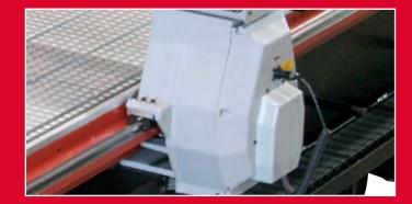
The steel gantry runs on high-quality linear bearings and is driven on both sides by servo motors coupled through planetary gearboxes. This provides a strong transmission for quality high-speed machining and auto-squaring of the gantry for precise alignment at all times.
