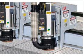
The twin-carriage option allows two parts to be cut simultaneously, effectively doubling production capacity and enabling faster job turnaround.
