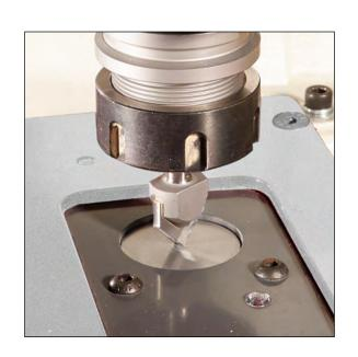
The tool-length sensor is used to automatically measure the length of a tool and create an accurate tool-length offset. This time-saving feature ensures precise and consistent cutting depths with all tools.
