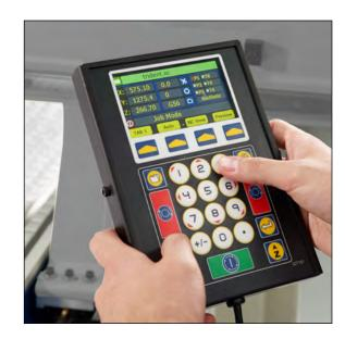
The AXYZ SmartConsole brings unprecedented ease of use, context sensitive menus, real-time display of machine status in addition to many more time-saving, functional and productivity features. It provides a graphical preview and current status of a running job and allows program feeds and speeds to be changed without pausing the program.
