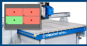
The industry exclusive Live Vacuum Bed technology is standard on every machine with automatic vacuum zone switching to ensure optimal holding power. Auto-zone management allows the router to operate in Live Bed mode, automatically activating and deactivating zones according to the live position of the cutting head.
