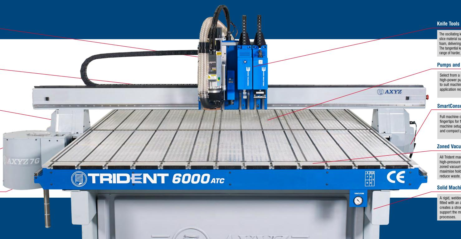
The oscillating knife will easily slice material such as soft or hard foam, delivering clean-cut edges. The tangential knife can cut a range of harder, heavier materials
