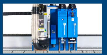
Processing a wide range of materials requires more than one cutting head. The Trident combines three different cutting technologies to provide maximum versatility by offering a choice of routing spindle and two knives which can be either tangential or oscillating, or a combination of both.
