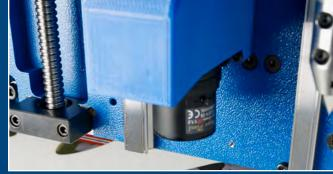
Additional options include an auto tool changer and the AXYZ AVS camera registration system. The AVS system quickly finds and recognises conventional registration marks to adjust the cutting path, providing exact alignment and 100% accuracy.
