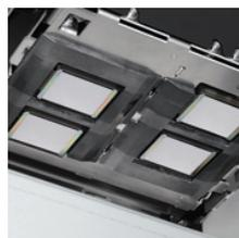
Dual staggered head setup / head height up to 4 mm
