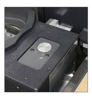
The tool length sensor is used to automatically measure the length of a tool and create an accurate tool length offset. This saves you time and ensures precise and consistent cutting depths with all tools.
