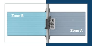
Pendulum processing allows truly continuous production by splitting the process area into two virtual zones so that a sheet can be processed on one zone while parts and waste from the other are removed.
