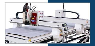
Dual gantries on a single machine bed offer a compact and cost-efficient alternative to purchasing two router tables. The independently driven gantries allow simultaneous processing of the same or different jobs even with different tools on both ends of the table.
