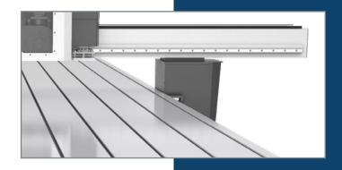
For applications that need a greater vertical clearance such as mold making or three dimensional carving, the standard 150mm gantry height can be extended to 250mm, 300mm or even greater.
