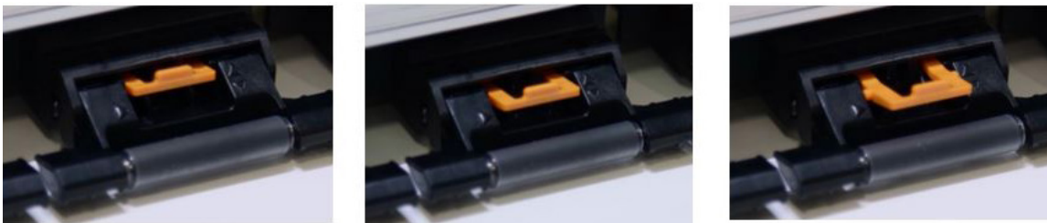
Adaptable pressure modes aid media feeding
